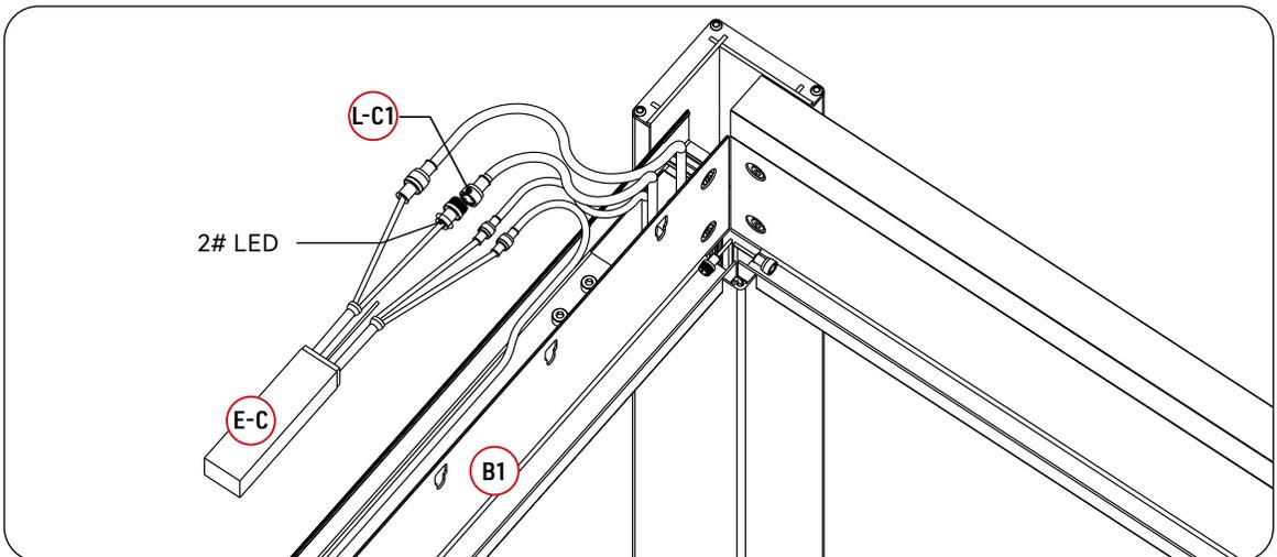
Install all LED strip in series, then connect the two ends of the LED strip with the two output line of the LED Controller(L-C1)
