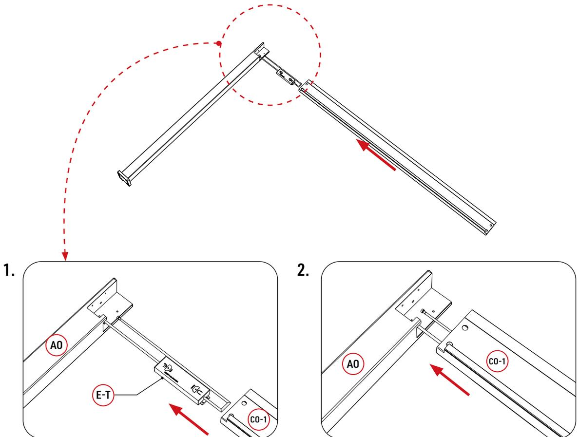
Connect the beam(CO-1) with the post(AO) as the diagram shown below.
