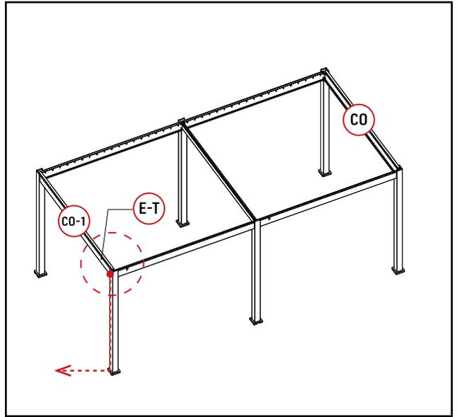
Insert the transformer into the cavity of CO-1, please note to reserve enough length of the power cable
