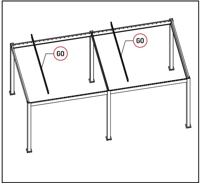
Install the the MAIN louver on the beam
