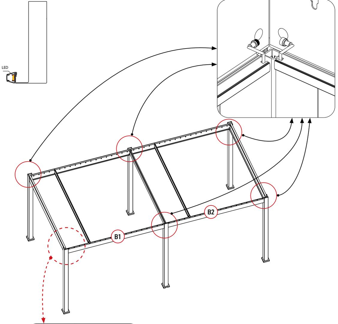
Insert the LED strip into the gutter, then connect it with LED Controller
